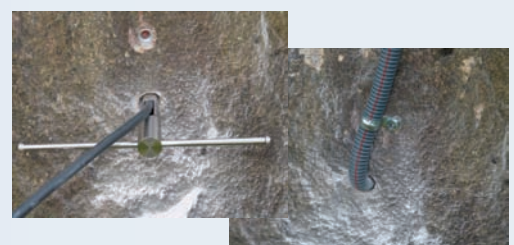
Figure 4) PERMASENSE node within weatherproof enclosure and protective housing mounted around Sphinx on 3550 a.s.l. Battery supply is sufficient for at least one year autonomous logging and communication. Snow covered nodes store their data and transmit as soon as they have contact to other nodes, again.
