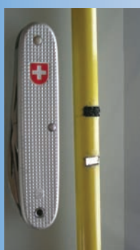
Figure 4) 14mm sensor rod with conductive foam electrodes. A thermistor on the reverse side measured temperatures.
